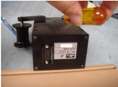
One set-screw to secure auxiliary roller
