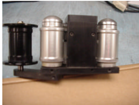
Two set-screws to secure rollers
