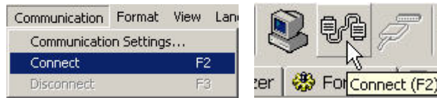
Figure 3-2. Select Connect from the Communication menu or click the Connect icon.
