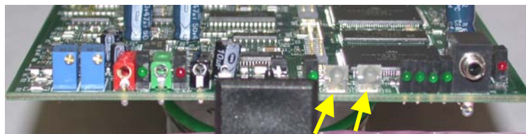
Figure 3-5. The two green LEDs will illuminate when level is correct.
