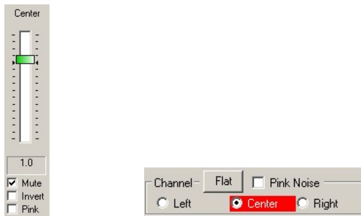
Figure 4-28. When channel is muted in Outputs, it will be highlighted in red in Equalizer.
