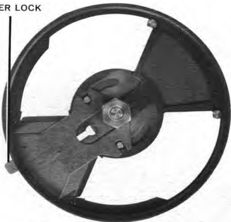
SUPER-40 SHUTTER IN 2-BLADE POSITION
