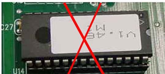
Installing the IC backwards will damage it!
