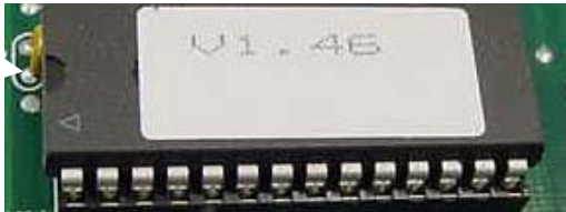
Install new U14 in D422. Verify pin 1.
