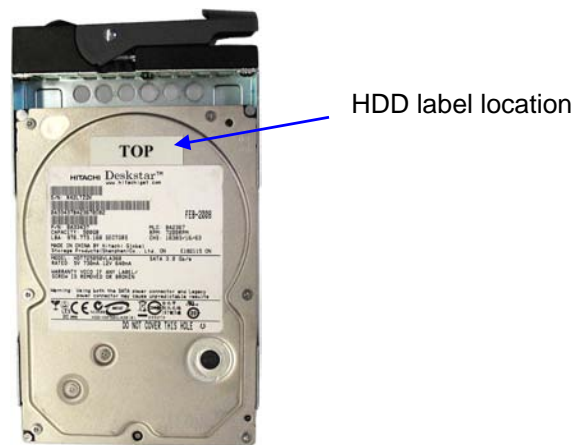
Figure 1: HDD Label Location – Example of “TOP” label
