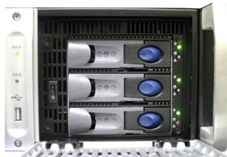
Figure 6: SMS-2K-1 Front Panel, Right Door Opened - Three HDDs
