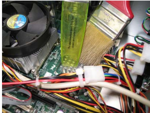
Figure 12: Motherboard Northbridge Heatsink Cleaning
