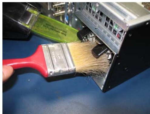
Figure 11: PSU External Fans Cleaning
