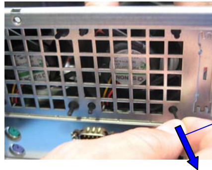
Figure 21: 2U Fan Shock Mounts Re-attachment Example
