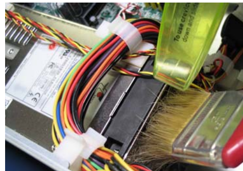
Figure 10: PSU Big Fan Cleaning
