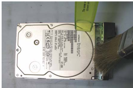
Figure 17: Hard Disk Drive Cleaning
