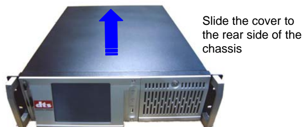
Figure 6: Digital Cinema Server - Lid Removal
