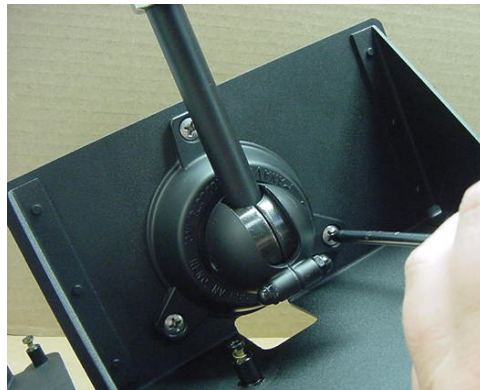
Figure 2. Secure mounting foot to EMA chassis.
