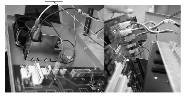
O Use the saved screws to connect the new rear panel and plug in all internal boards.
