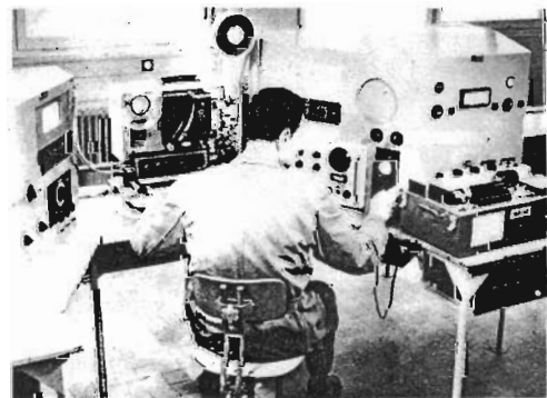
Checking the sound quality of an S-221 projector electronically.
