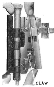
CLAW REPLACING RUNNER
