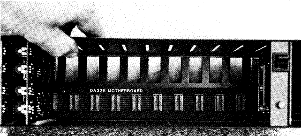
INSIDE VIEW OF CARD CAGE SHOWS THE MOTHER BOARD WITH CONNECTORS FOR ALL PLUG IN CARDS.
