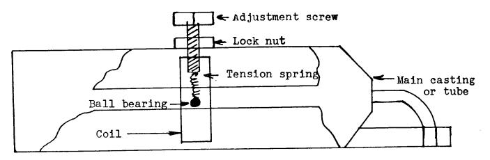
If at any time it is necessary to remove the armature rod that extends through the center of the coil, care should be taken to REMOVE THE BALL BEARING AND TENSION SPRING FIRST.
