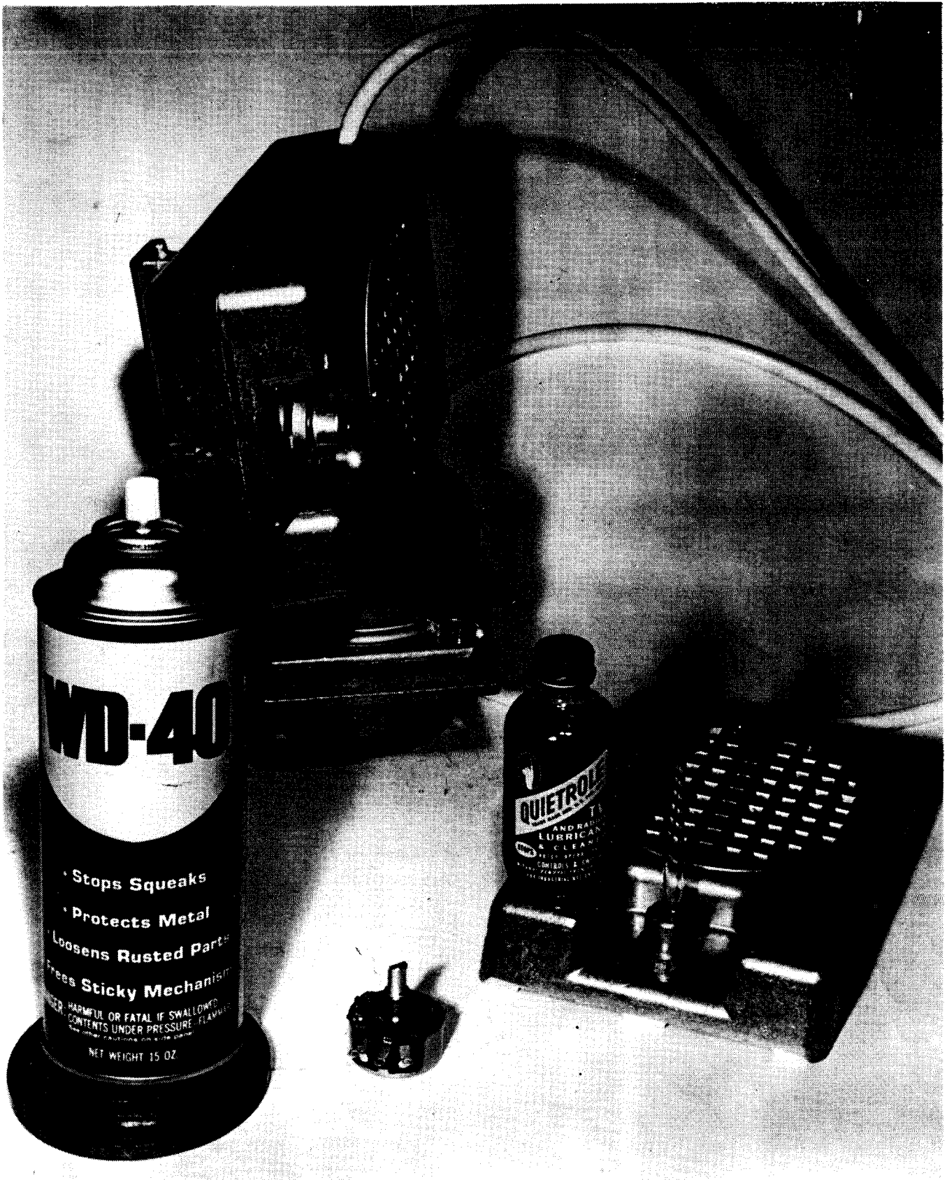
WD-40 and Quietrol for treating noisy Volume Controls. The tube supplied with WD-40 is positioned through the slot of Reed Speaker so that it is over the terminals of Volume Control. Squirt and work Control back and forth. Quietrol may be applied through the #155 hole, work control up and down and back and forth.
