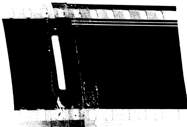
Never use ordinary tapes (such as the Scotch tape shown here) for making film splices.
