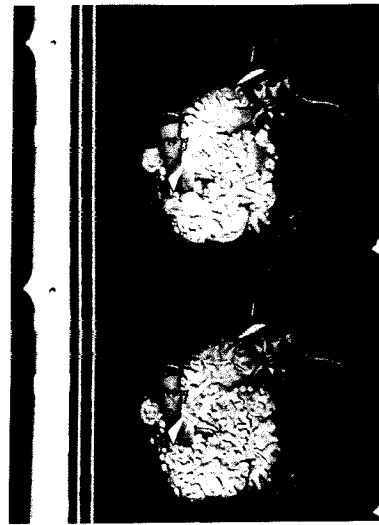
Blistered films such as this must be thrown out, but blistering can be prevented easily by proper adjustment of the lamphouse.
