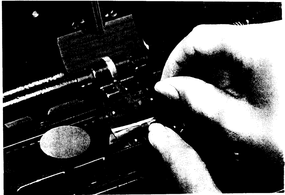
Figure 6. Small weights or magnets permit two-hand operation.
