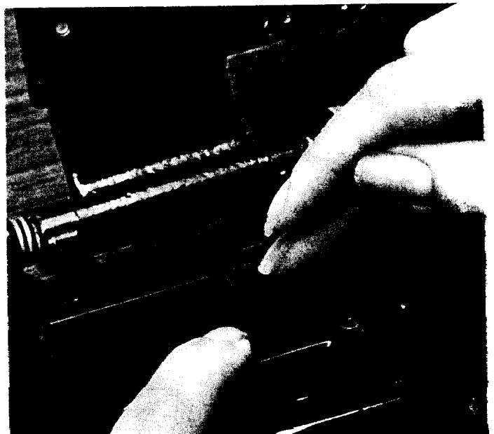
D. Smooth out finished splice.
