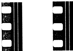
Black optical soundtracks, left, were replaced with "high-magenta" tracks, right.
