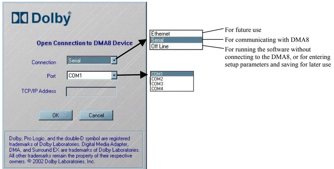
Figure 3-1 Open Device Screen
