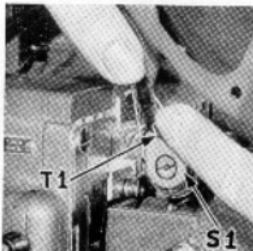
below sprocket S1. Slide the film as far toward the machine as it will go. Holding the film snugly around the sprocket with the right thumb and index finger, press on tab T1 to open the guard. Pull gently on the film until the perforations seat on the sprocket teeth.
