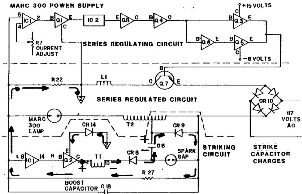
The high output from pin 14 of (IC1) turns transistor (Q2) fully on so the high voltage winding (F-D) of auxiliary transformer (T1) can charge the strike
