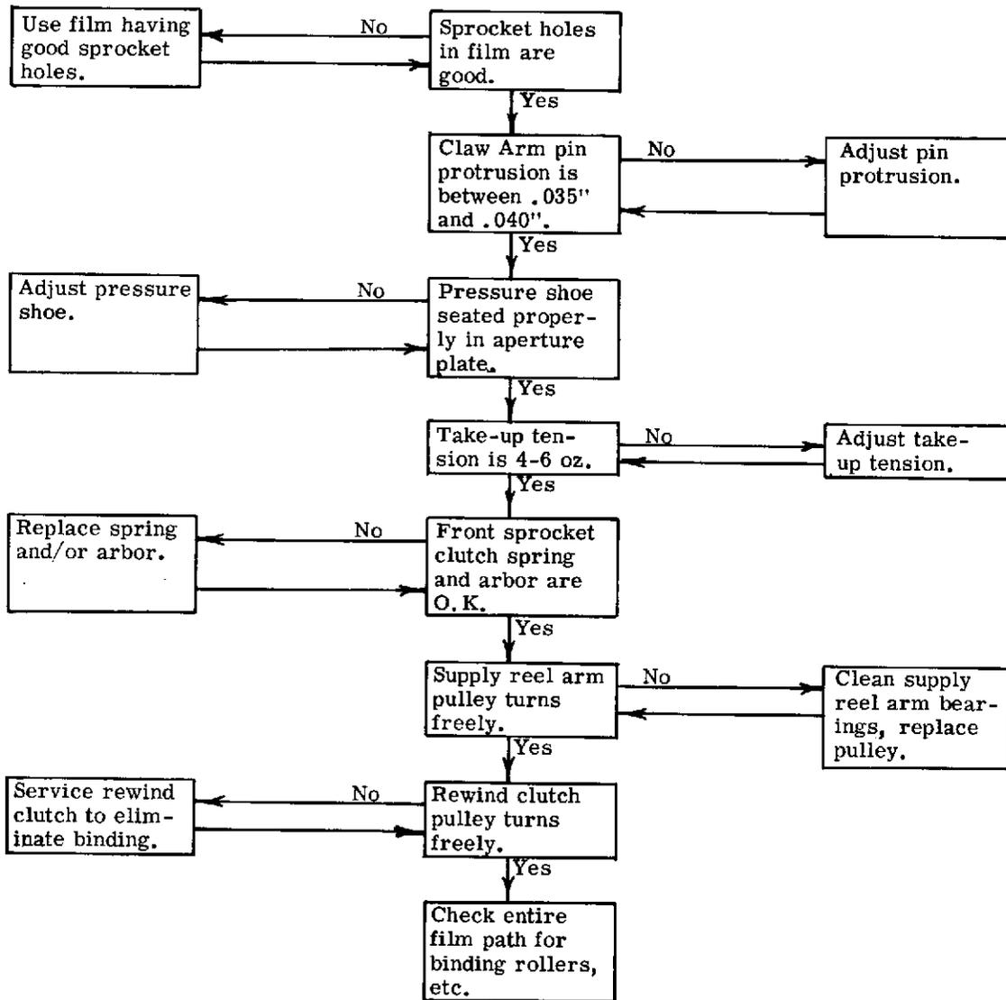
**Auto Loop Restorer Cycles Continuously**
