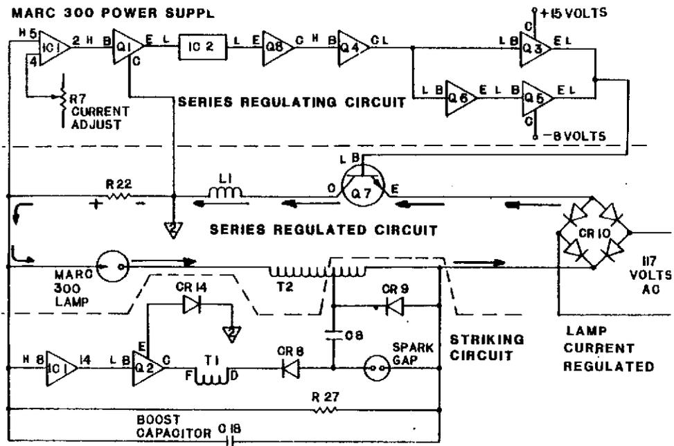
A voltage appears across Resistor (R22) which causes a high to appear at pins 5 and 8 of (IC1). The high output from pin 2 of (IC1) conditions the series regulating circuit to drop the voltage on the base of (Q7) so it will regulate current in the series regulated circuit to 7.7 amps as preset by resistor (R7). The low output from pin 14 of (IC1) turns transistor (Q2) off and disables the strike circuit.
