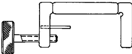
Used to hold solenoid while setting stroke.
