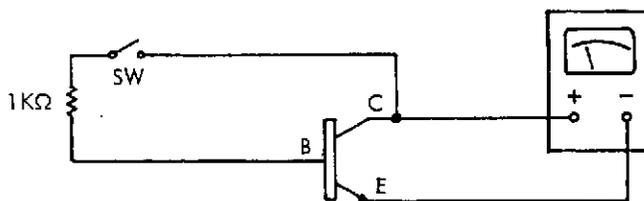
Use the X100 scale for regular small-signal devices and X10 scale for power types. All readings are referred to the X1 scale.
