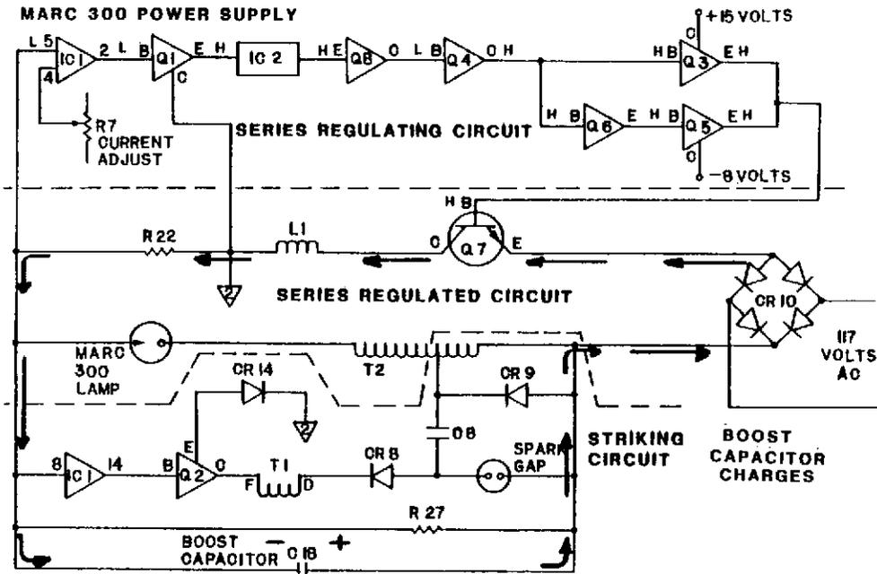
The low output from pin 2 of (IC1) conditions the series regulating circuit to turn Transistor (Q7)
