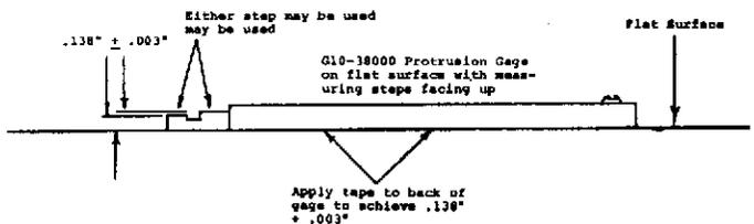
If neither step measures  $.138 \pm .003$ ", build up the back side of the gage with tape until the correct thickness is obtained.
