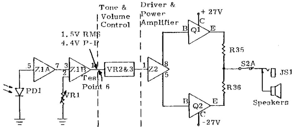
Figure 5-1. 16mm AUDIO AMPLIFIER-BLOCK DIAGRAM
