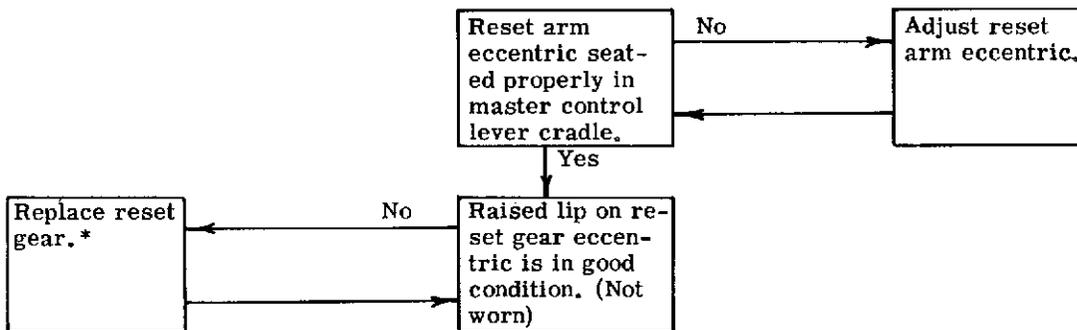
\* If the gear eccentric is worn, carefully examine the latch tab on the Loop Resetting Arm for rough edges or burrs.
