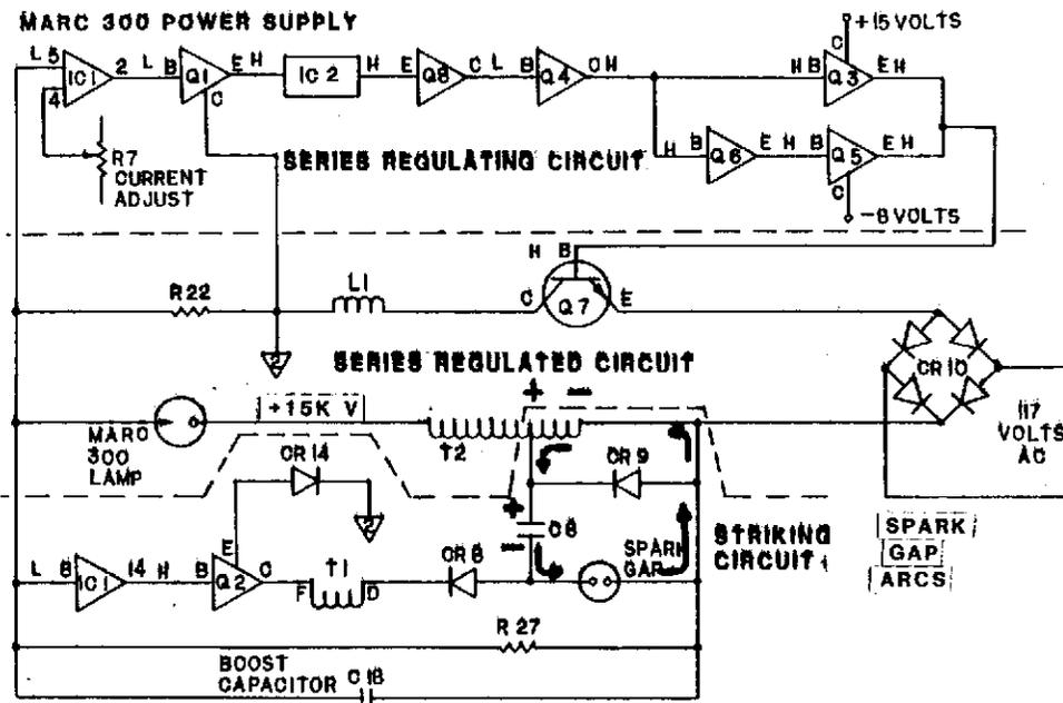
When the spark gap arcs, (C8) discharges through the primary winding of pulse Transformer (T2), which
