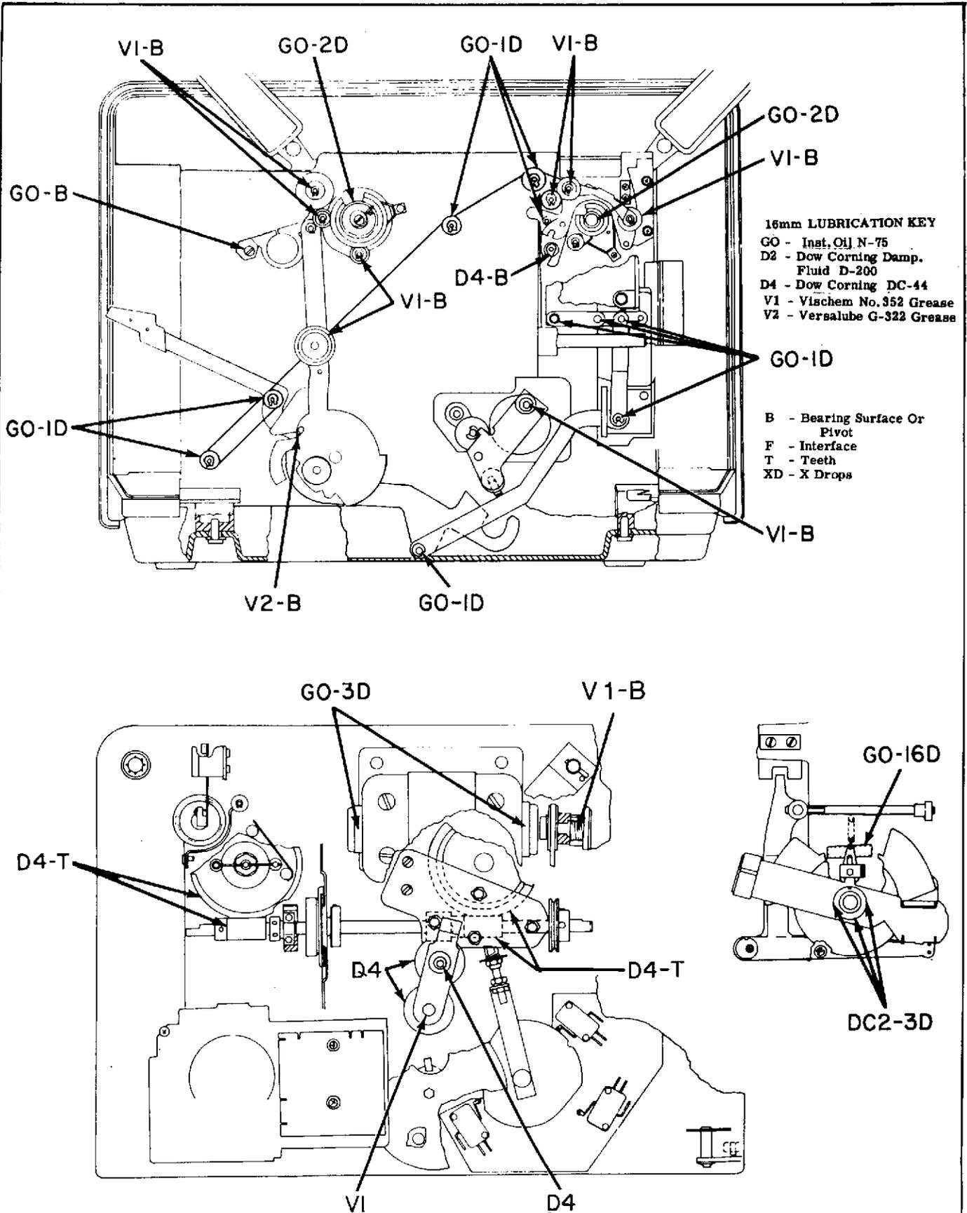
Figure 3-46. PREVENTIVE MAINTENANCE LUBRICATION POINT DIAGRAM
