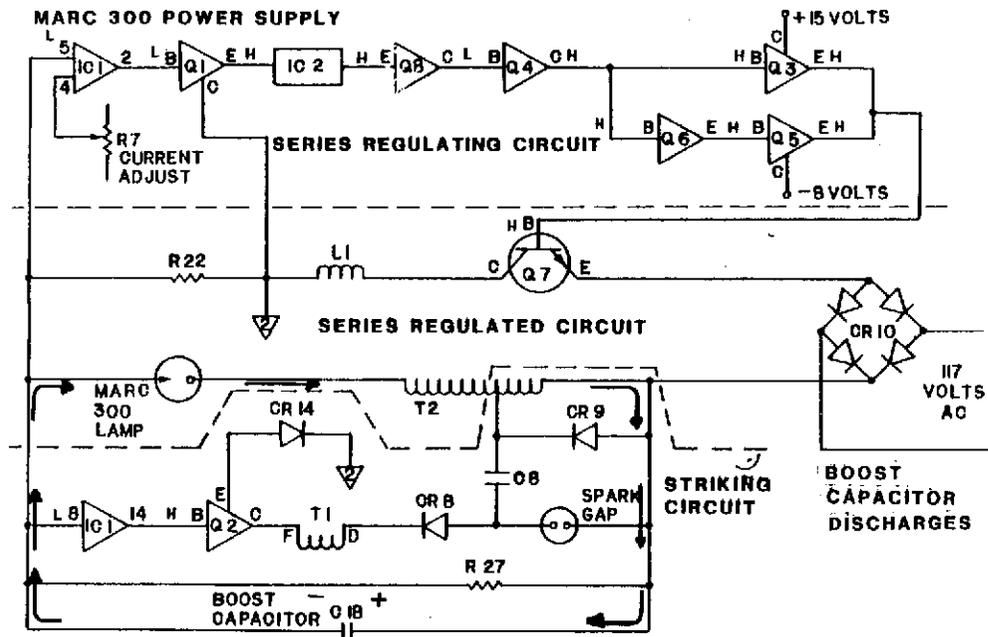
The Arc Lamp ignites and the boost Capacitor (C18) discharges through it to sustain conduction long
