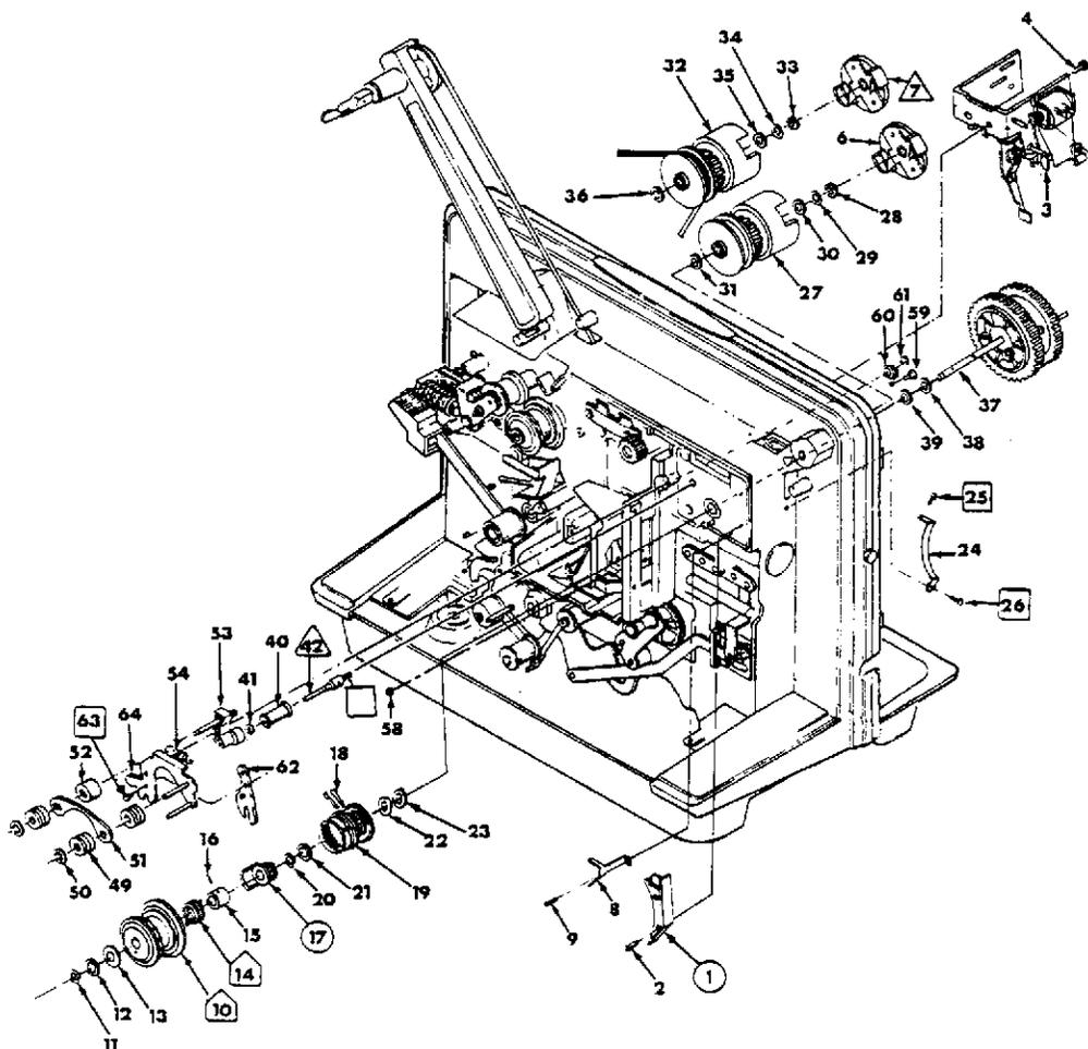
Figure 3-2. REMOVAL AND REASSEMBLY OF FRONT CLUTCHES
