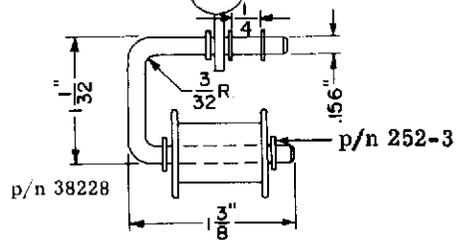
Used to measure forward take-up tension, belt tension and fast forward take-up tension. The scale reading is twice the actual film tension.
