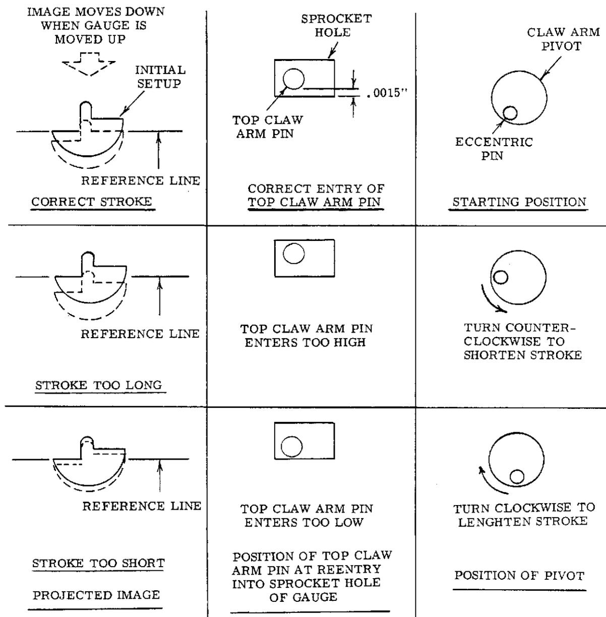
9. If the stroke was adjusted, repeat Steps 3 through 8. When performing Step 6, it is quite probable that the bottom step of the projected Target no longer rests on the reference line. ADJUST THE ELEVATION to line up the bottom step of the projected Target with the reference line and then proceed with Steps 7 and 8. It may be necessary to repeat this sequence of steps several times until correct stroke and side clearance are obtained.
