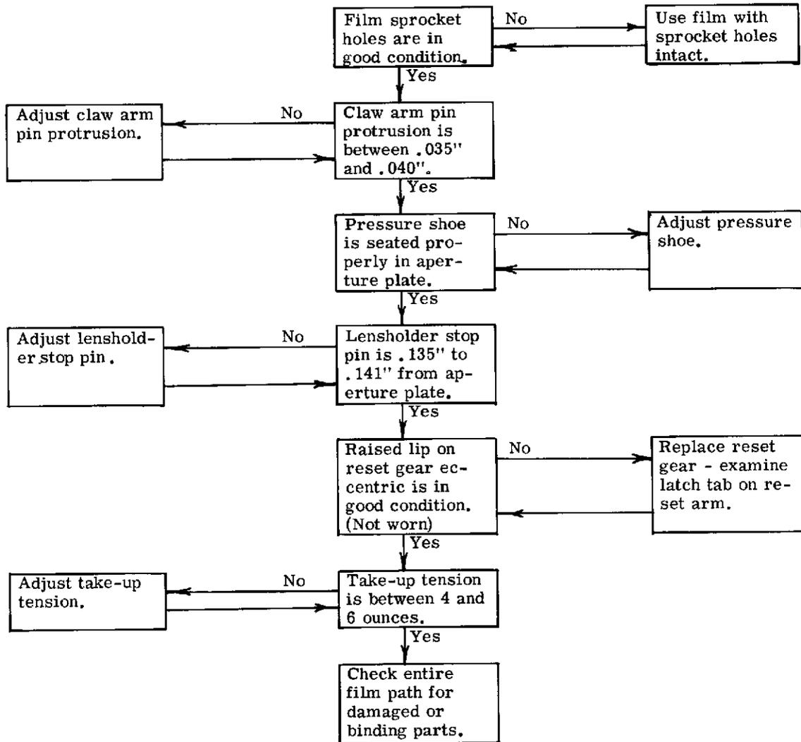
**Auto Loop Restorer Recycles Continuously In Fast Forward**
