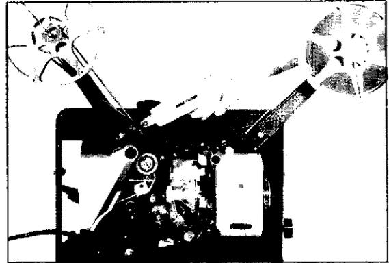
Adjust the take-up tension adjusting nut up to increase tension and down to decrease it.
