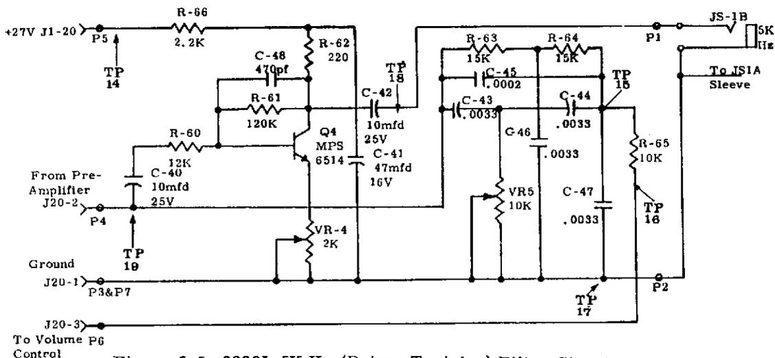
Figure 5-5. 2220L 5K Hz. (Driver Training) Filter Circuit
