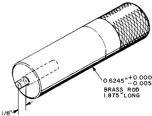
Used to locate the lateral and rotational position of the sound drum.
