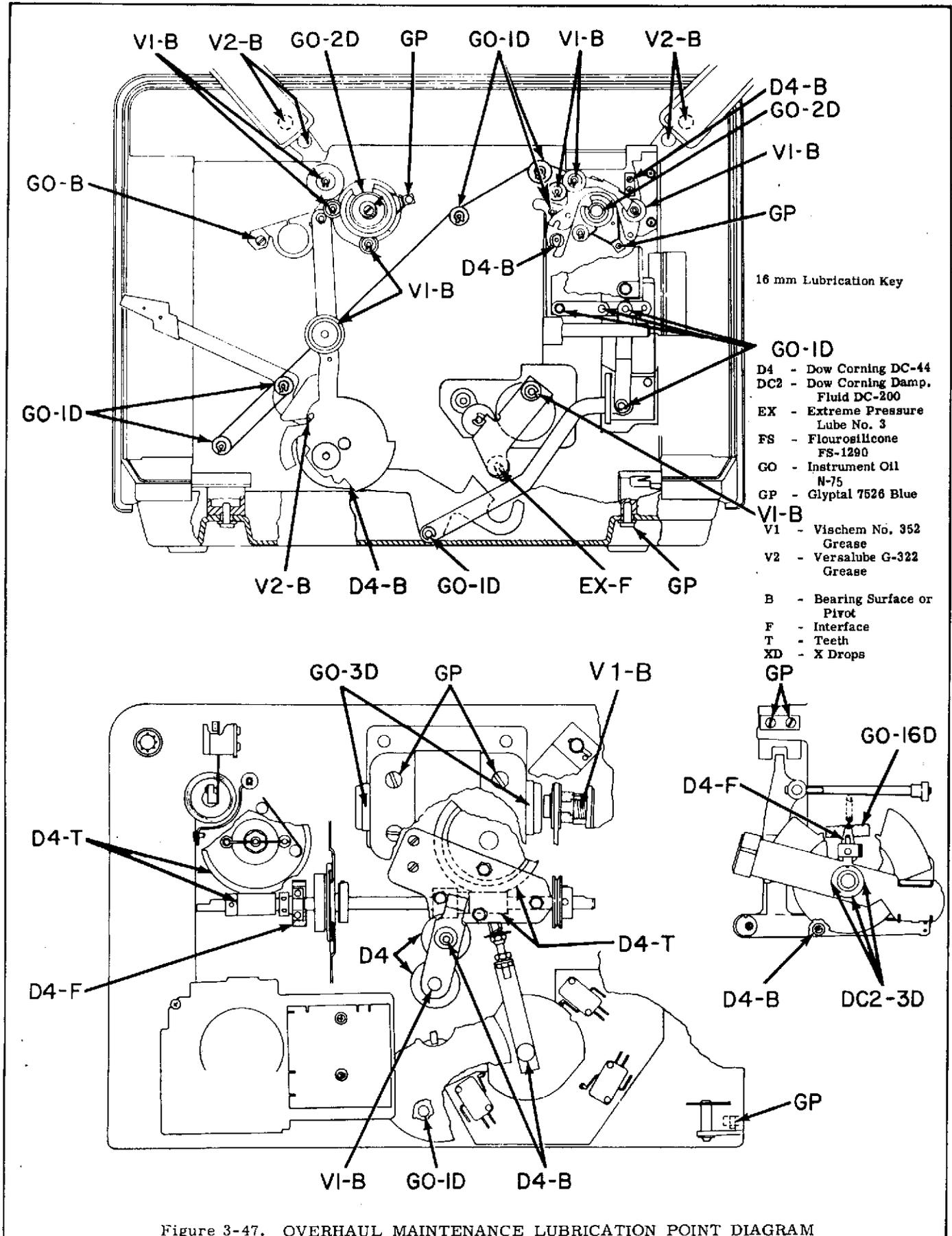
Figure 3-47. OVERHAUL MAINTENANCE LUBRICATION POINT DIAGRAM
