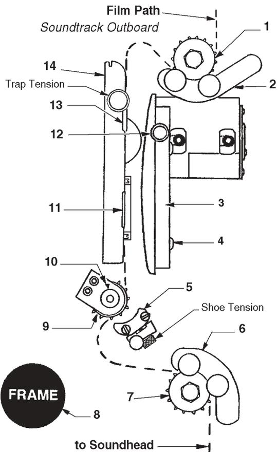
Unlatch and open the turret. Rotate the framing knob (Item 8) to its center position (FRAME reading level, as shown). Using the soundhead flywheel, turn the mechanism by hand to rotate the intermittent sprocket (Item 9) to its "rest" position. In the "rest" position, the index mark (Item 10) will align with one of the painted white index lines on the intermittent shaft collar after the sprocket has completed a four-perforation step.
