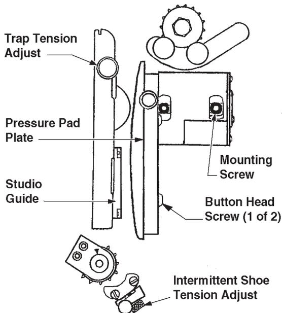
1. Open the turret. Dismount the gate pressure pad runner by removing the two 10-32 button head cap screws using a 1/8 inch right-angle allen wrench.
