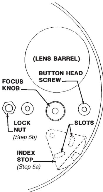
5. Periodically check lens positions and correct as required. Project RP-40 Test Film to the screen and alternate between formats. If the picture shifts up and down, or left to right between formats, the lenses must be re-positioned.
