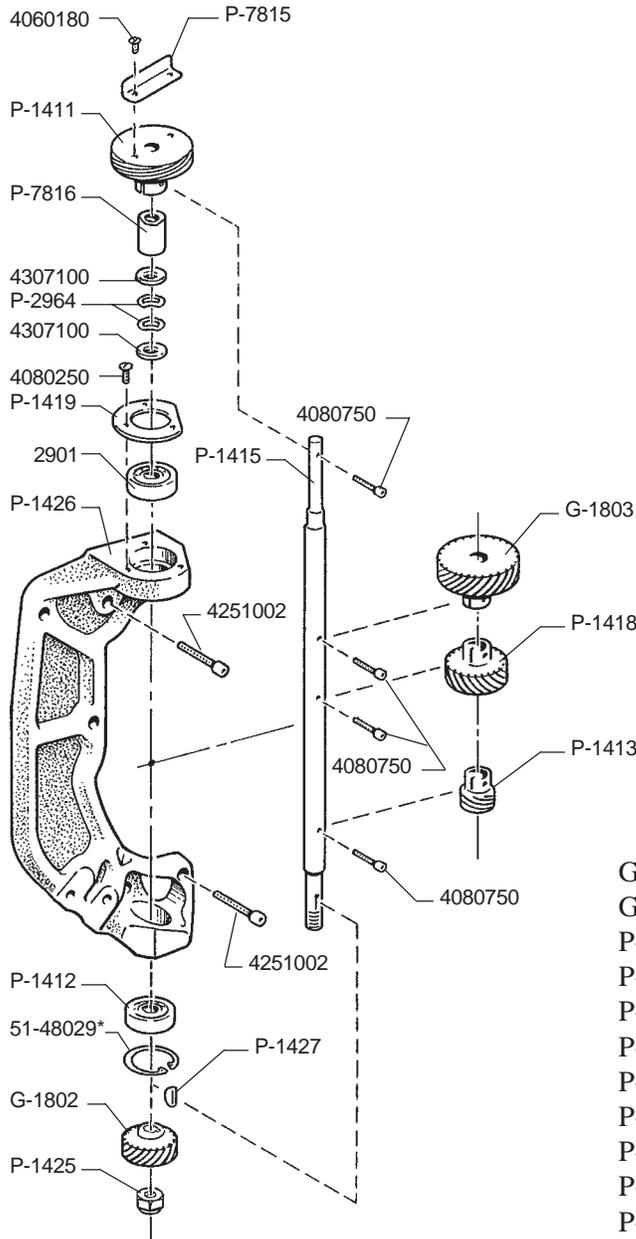
\* Install Snap Ring with beveled side down
