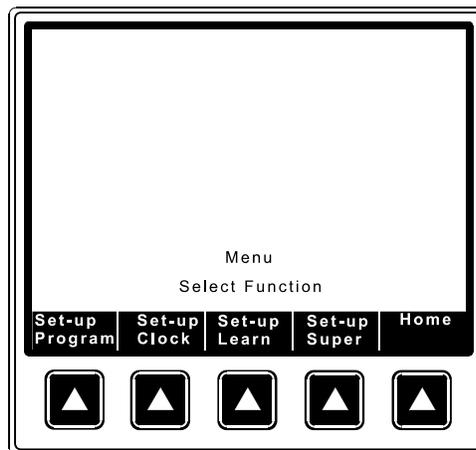
Figure 2.41: From the Set-up screen press [Set-up Clock].
