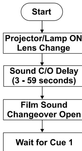
*Cue (with a lens change).* At the cue the changeover is closed, sound is muted and the lens is driven to it's new state. After the lens changeover time , the changeover opens and the film sound is selected. The lens changeover time can be programmed from 0 to 9 seconds.
