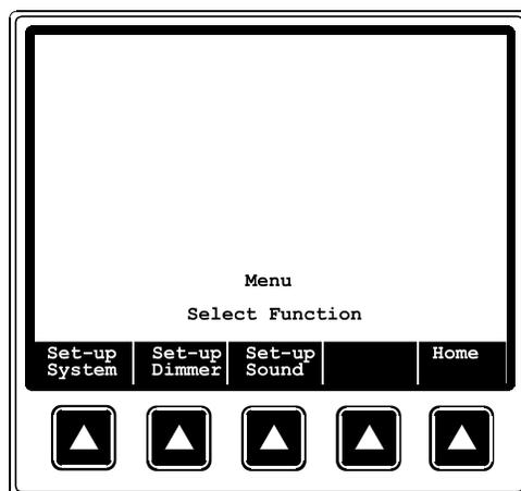
Figure 2.18: Press Set-up Dimmer.
