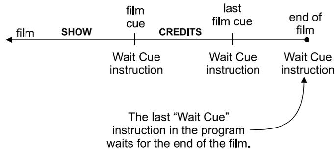
\*The projector motor shuts off at the end of the film.
