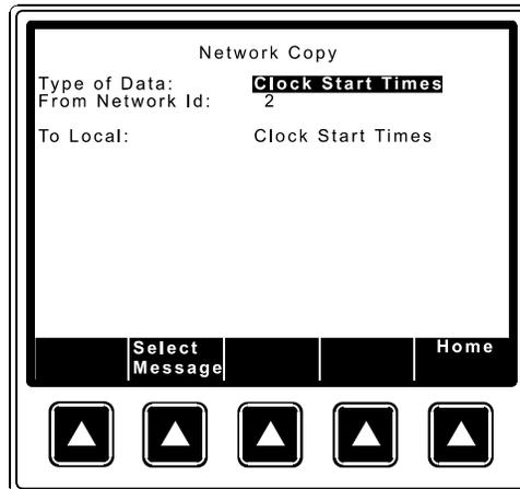
Figure 2.55: Enter the Network Copy screen and select the “Type of Data” to be copied.
