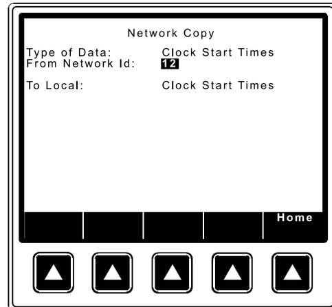
Figure 2.56: Cursor to the “From Network Id” field and enter the Id of the CNA-200 you want to copy data from.
