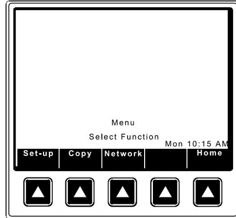
Figure 2.25: Press the [Set-up] key to go to the set-up menu.
