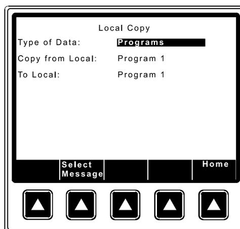
Figure 2.50: Select "Type of Data" to copy by pressing the [Select Message] key.
