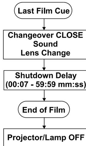
There are a two ways the CNA-200 can end a show. The *film run-out* method is the most typical way to end the show. Insert a Wait Cue instruction at the end of the program. (Do not put a cue on the film.) The shut down sequence will begin when the end of the film is encountered.
