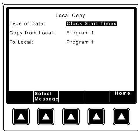
Figure 2.49: Press [Local Copy] and enter the high level password.
