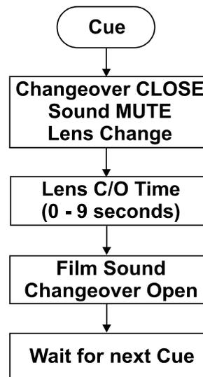
*End of Show Sequence (with format instruction).* When the last film cue is encountered, the changeover closes and sound and lens are driven to their new state. The shutdown delay has a programmable range of 7 seconds to 59 minutes:59 seconds.
