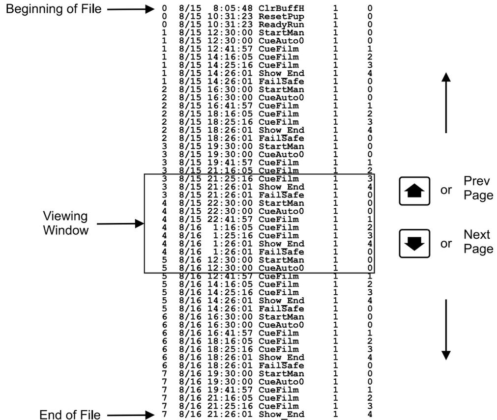
This shows how the CNA-200 moves through and displays the Event file.
