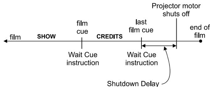
\*The projector motor shuts off when the timer expires or the end of the film.
