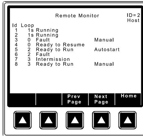
Figure 2.62: Press the [Network] from the Main Menu. Press [Remote Monitor].
