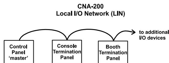
The LIN will also support devices such as dimmers, failsafes, auxiliary control panels and automatic volume control. The LIN is designed to support up to 32 devices.
