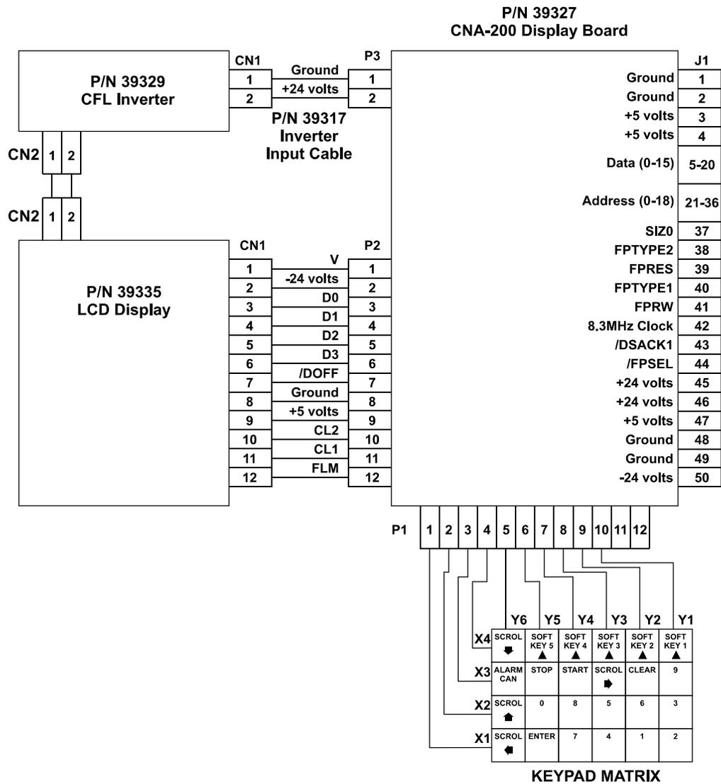
CNA-200 Keyboard and Display Block Diagram
