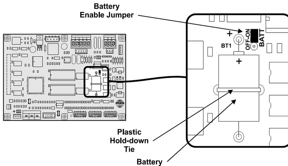
CNA Battery Jumper Configuration
