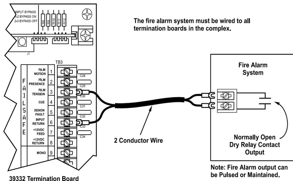
Fire Stop Input Wiring
