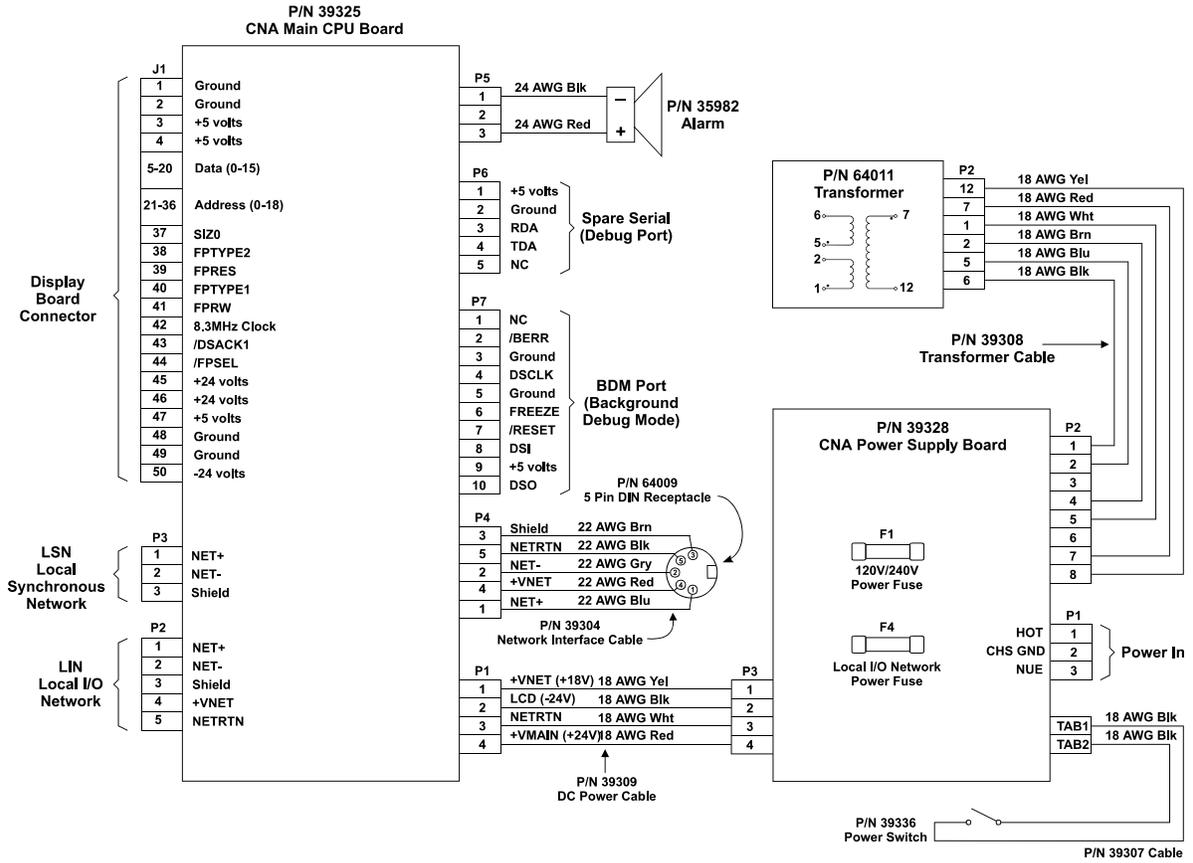
CNA Main CPU Board and Power Supply
