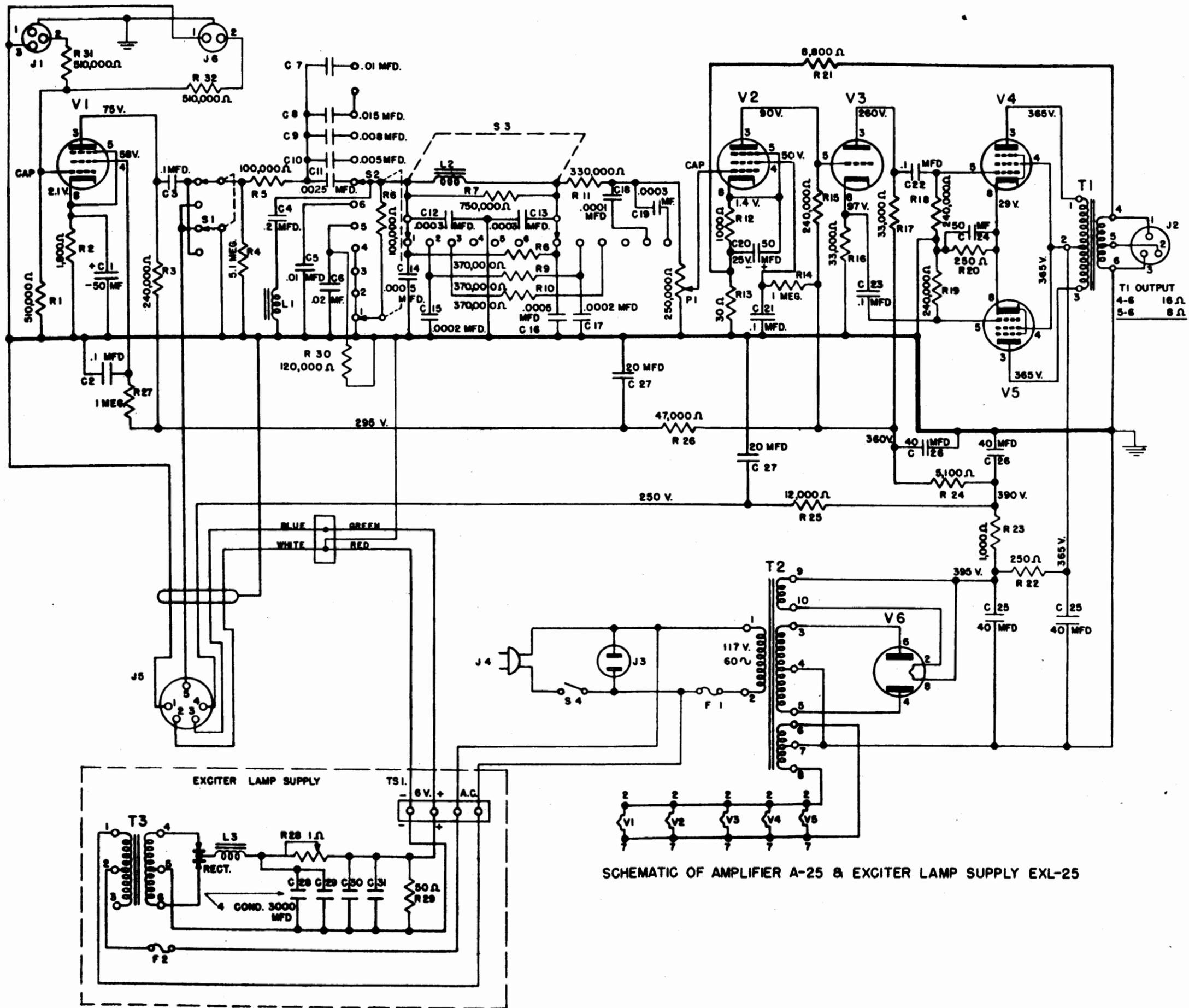
SCHMATIC OF AMPLIFIER A-25 & EXCITER LAMP SUPPLY EXL-25
