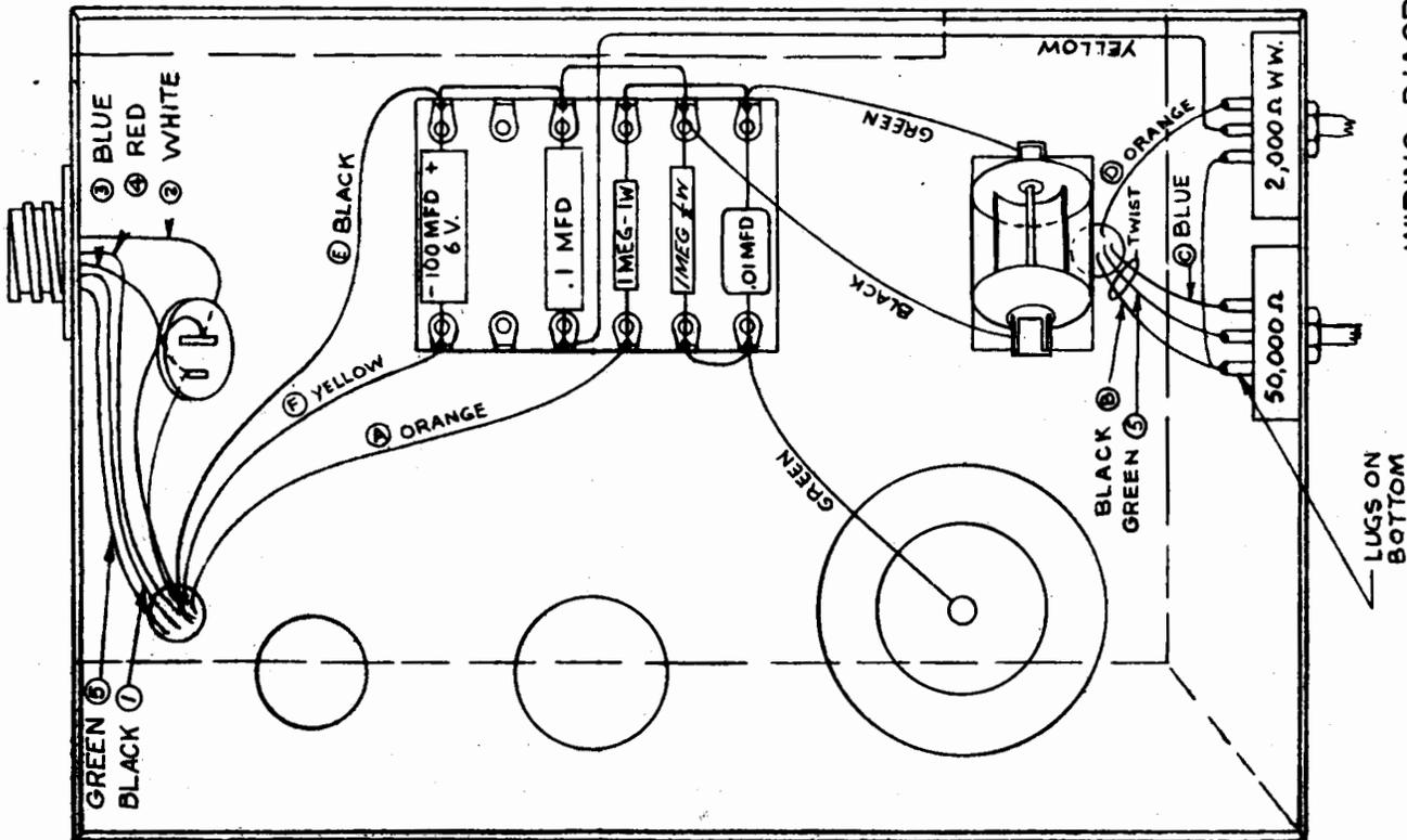
WIRING DIAGRAM OF PRE-AMPLIFIER PRE-25
