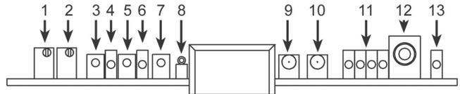
6. If the left indicator (9) is red, the signal is too low. Rotate the main fader control clockwise to raise the level. When the level is correct, the indicator (9) will turn green. A flashing red means that the signal is too high.
