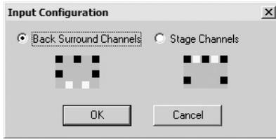
The processor supports either five screen channels or “Ex” back surround channels but not both.
