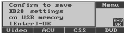
Insert the USB memory device into the USB port on the XD20 and press **Enter** to start. Press **◀** to abort. If there is no USB memory device connected to the XD20, a message appears and asks you to insert one.
