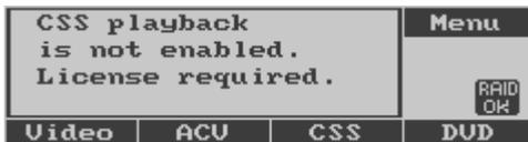
If XD20 is not equipped with the CSS Option, the CSS Playback menu will be locked.
