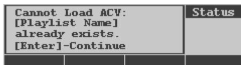
The following message appears if the content cannot be loaded due to space limitations. In the example shown, the system ran out of disc space part-way through the playlist named
