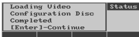
4. Press **Enter** and the disc trays will open. Remove the disc from the tray.
