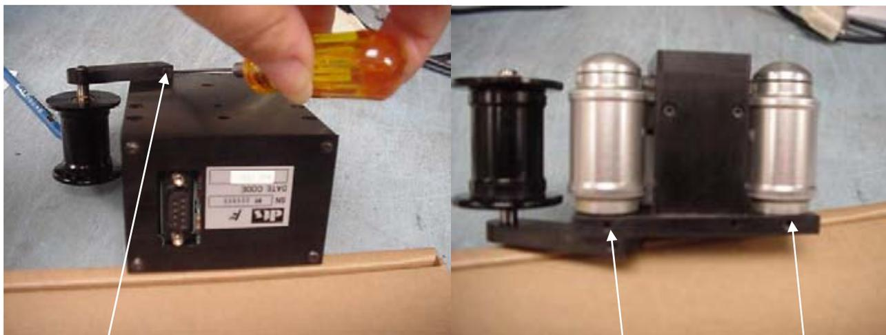
One set-screw to secure auxiliary roller
