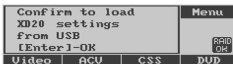
Insert the USB memory device that contains the settings for your XD20 into the USB port and press **Enter** to copy the settings onto the XD20’s hard drive. Press **◀** to abort. If there is no USB memory device, a message appears, asking you to insert one.
