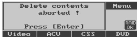
**Yes** Delete all soundtrack and CSS content files for the selected feature. A *Delete in progress* message will be displayed while the content is being deleted.
