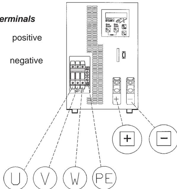
After having performed the cable connection, take in place the protective plate (see directions on next page).
