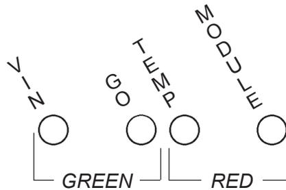
WHEN BOTH of the green indicator lights are glowing, the power supply is operating normally and trouble-free. A red light, when glowing, indicates that a problem exists, and disables operation of the power supply.
