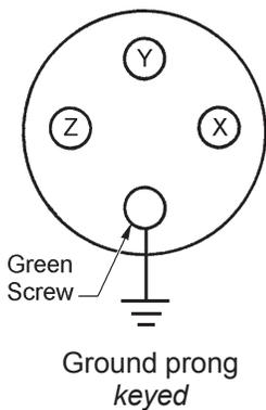
A four-prong, female plug is furnished to mate to the AC receptacle mounted to the power supply. Connect 208/230 V.AC three phase input to terminals X, Y, and Z. Connect single phase input to terminals X and Z *only*. Single or three phase neutral is not required for installation of this unit. Attach an adequate earth ground to the green ground terminal.
