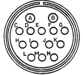
Modification for use with Spotlight or other non-console lamphouse: Remove the jumper from between Pin E & F; remove black lead from Pin C and relocate to Pin F. This will supply 110 V.AC to the main board for the **GO** light.
