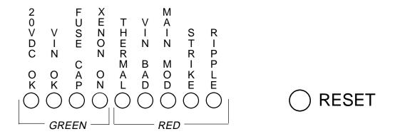
WHEN ALL FOUR of the green indicator lights are glowing, the power supply is trouble-free and operating. One or more red lights, when glowing, indicates that a problem exists, and disables operation of the power supply. The red light(s) latches and remains glowing until the RESET button is depressed after correcting the problem.
