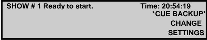
The next time the show is run it will be under the close scrutiny of the Cue Backup feature, so that if a cue is not seen by the appropriate sensor the 'Cue Backup' will generate the cue anyway.
