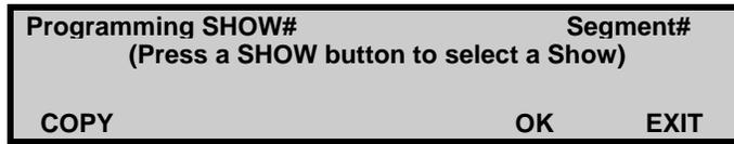
Select the Show that you wish to copy using the Show # keys and then press the **COPY** softkey. An extra softkey function called "PASTE" will appear. Select the Show # that you wish to paste the information into using the Show # keys and press the **PASTE** softkey, this can be repeated to as many Shows as necessary.
