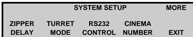
Press the **ZIPPER DELAY** softkey, the volume display will change to dashes to indicate that the control is in SCROLL mode and the screen will change to:
