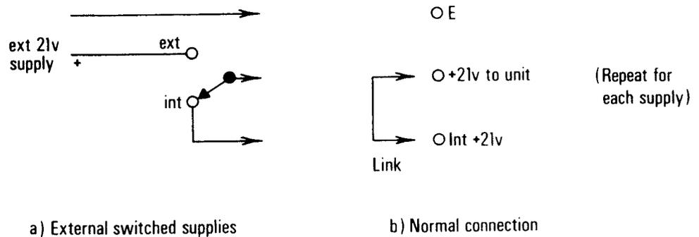
The precise values of the external voltages are not critical, except that they should be within the ranges  $\pm 2$  volts on the 15 volt supplies and  $-1, +3$  volts on the 21 volt supply (the gain of the fader module is dependent on the absolute value of the 21 volt supply, and if a somewhat different value is used, it may be necessary to alter the fader settings slightly).
