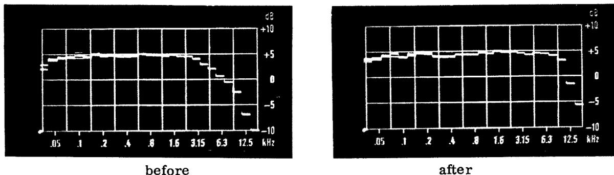
Fig. 7.6 Adjustment of Optical Pre-amplifier h. f. controls
