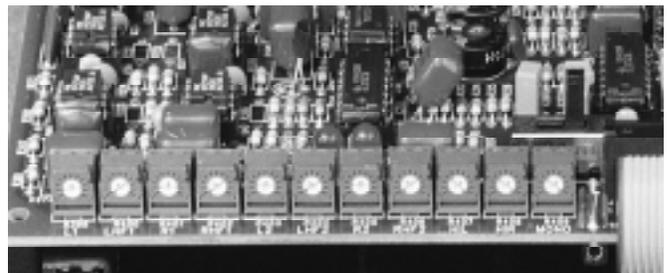
Figure 8. Left side potentiometers (Preamp, slit loss, hearing impaired, and mono levels) and preamp selection switch (SW1).
