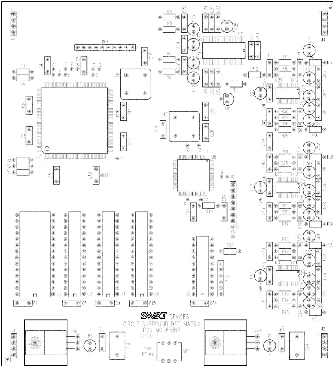
Figure 5a. MOD VI DSP Matrix circuit board diagram (left).
