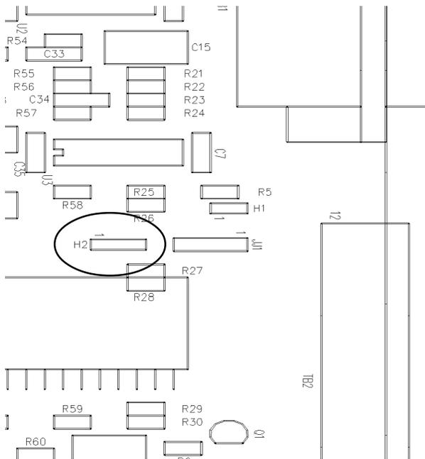
Figure 1. Enlargement of the H2 area of the Main circuit board. (Matrix board not shown).
