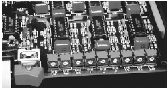
Figure 9. Right side potentiometers (Music, Digital, and main output levels) and Emergency Bypass switch (SW2).
