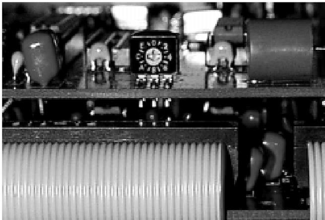
Figure 12. TIME DELAY rotary switch on the Matrix board.
