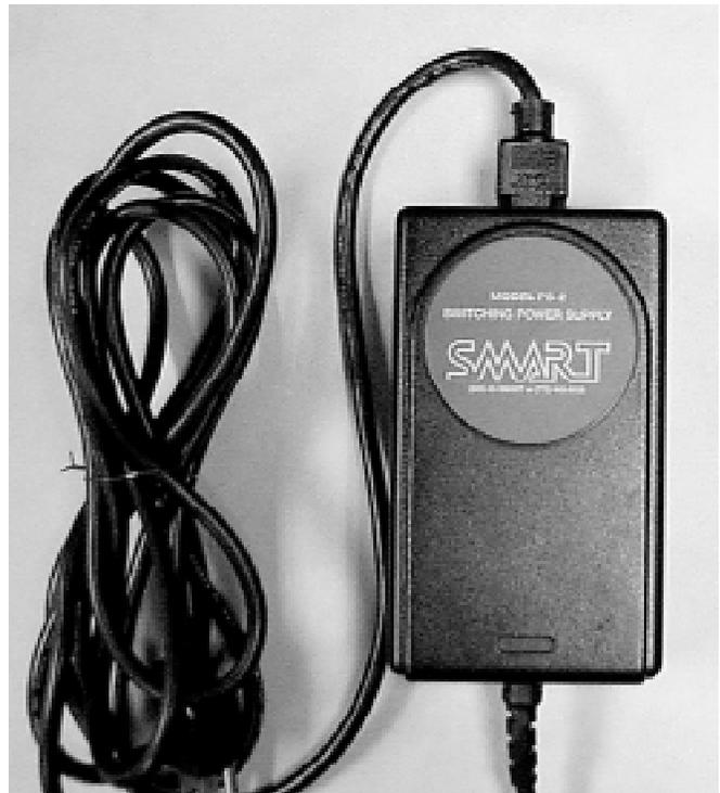
Figure 14. Model PS-2 switching power supply.
