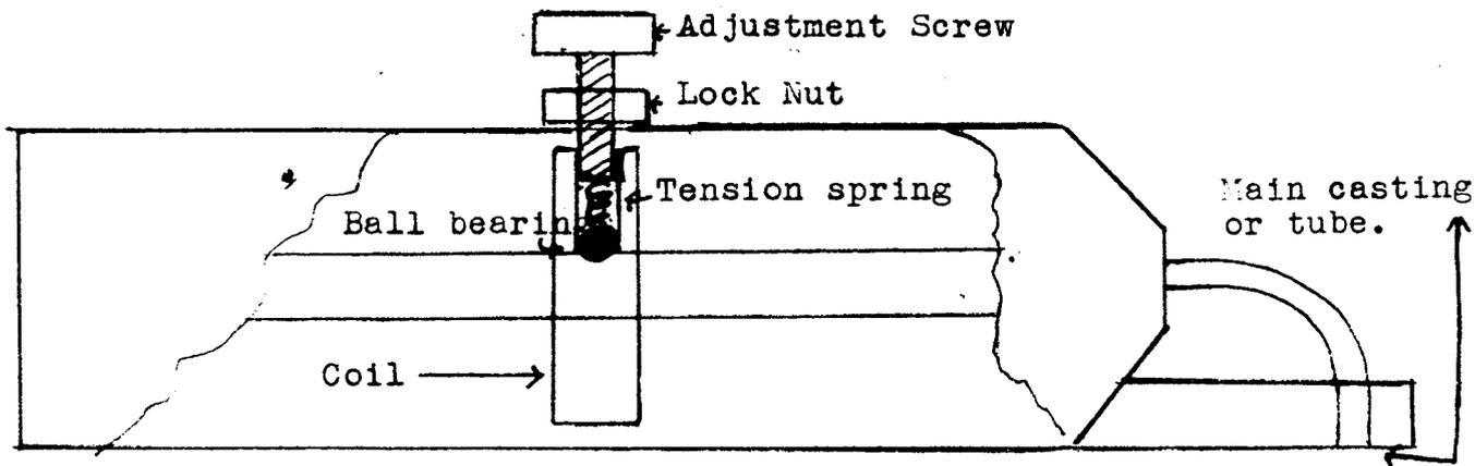
If at any time it is necessary to remove the armature rod that extends thru the center of the coil care should be taken to remove the ball bearing and tension spring first.
