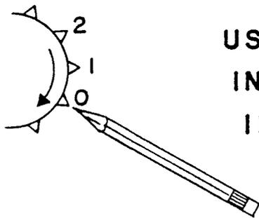
USE A POINTED OBJECT TO INDICATE POSITION OF INTERMITTENT TOOTH WHEN IN STOPPED POSITION.
