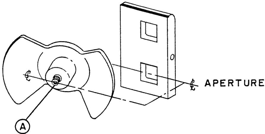
TURN PROJECTOR FORWARD BY MOTOR FLYWHEEL UNTIL SPROCKET TOOTH #2 IS AT INDICATOR. LOOSEN SCREW (A) AND TURN SHUTTER SO  $\mathcal{C}$  OF BLADE IS ON  $\mathcal{C}$  OF APERTURE OPENING.
