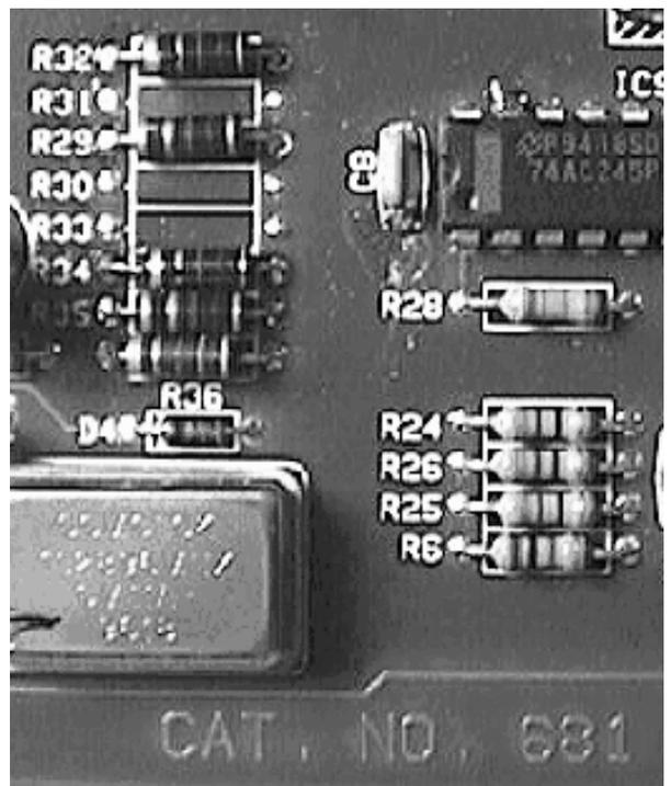
Note: The original resistors and the new inductors are similar in shape:
