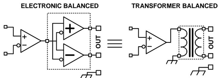
The circuit on the right uses a transformer to connect the output of an internal circuit stage to the outside world while isolating chassis ground from the audio signal. The circuit on the left uses a cross-coupled electronic circuit to achieve the equivalent result: true electronic balancing.
