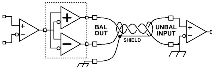
Once again the output signal must be properly terminated at the unbalanced input and the shield must be connected only at one of its ends so as to avoid connecting the two equipment grounds together and creating a ground loop. The cross-coupled circuit ensures that the signal level is properly maintained.
