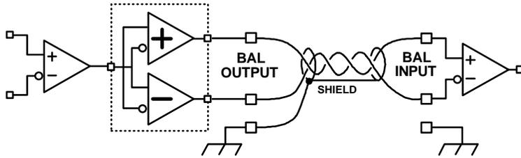
This circuit scheme gives the highest performance of all because it combines the benefits of balanced outputs with the even greater hum and interference reducing benefits of balanced inputs. It is the professional approach taken in the design of Sony cinema processors at both their inputs and outputs.
