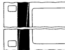
**Figure 7.** 35 mm Photographic Scanning Beam Test Film (SMPTE No. P35-SB).
