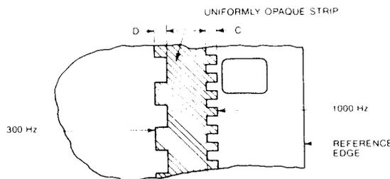
**Figure 6.** 35 mm Photographic Buzz Track Test Film (SMPTE No. P35-BT-400).
