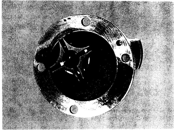
**Figure 5.** Partially disassembled Geneva movement showing the STARWHEEL.
